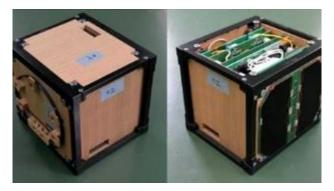
❖ In a world-first, Japanese researchers have built a tiny wooden satellite named LignoSat that will be launched into space on a SpaceX rocket.
